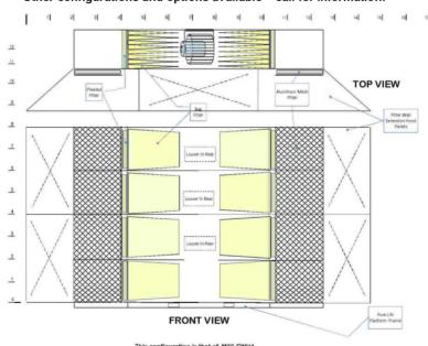
This configuration is that of M32-FWV4 unit contains (3) 110VAC 3/4hp motors
