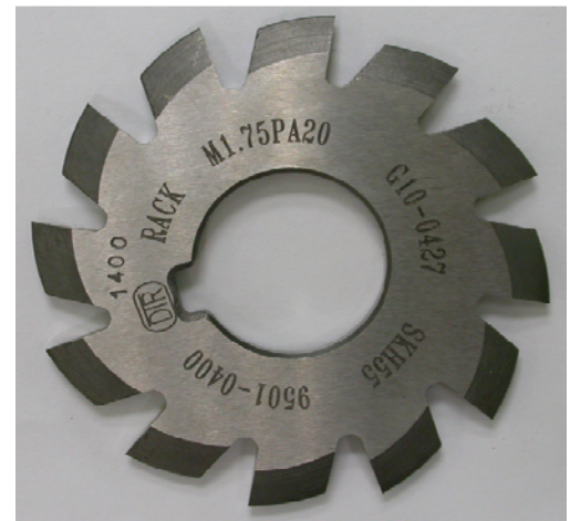
Nd:YAG Laser Marked, 1064 nm
